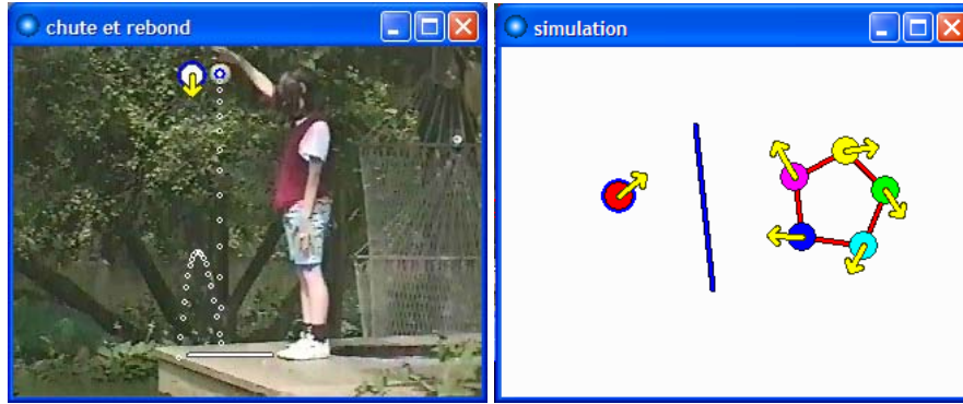
Figure 1: Examples of animation windows. In the window on the left, the points correspond to the positions of the real falling ball—the one on the right—as measured on the successive images of the video sequence—the ball on the left is a simulated one—. In the window on the right, three types of simulated objects are shown.
